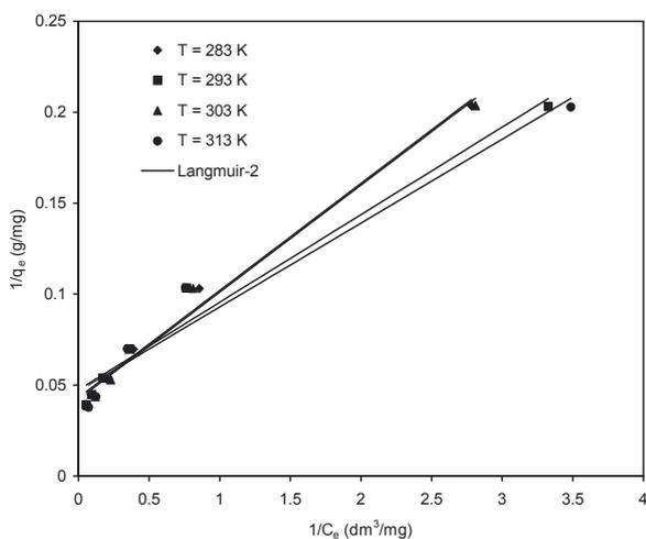
Fig. 2. Langmuir-2 isotherm obtained using the linear method for the adsorption of lead(II) onto peat at various temperatures.
