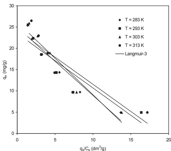
Fig. 3. Langmuir-3 isotherm obtained using the linear method for the adsorption of lead(II) onto peat at various temperatures.
