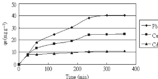
Figure 3. Adsorption capacities and equilibrium time for  $\text{Pb}^{2+}$ ,  $\text{Cu}^{2+}$  and  $\text{Cd}^{2+}$  adsorption on CCNTs.
