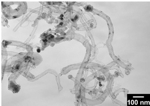
Figure 7. SEM image of CNTs/Fe-Ni with 20 nm TiO<sub>2</sub>.
