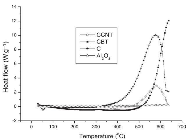
Figure 6. Comparison of heat flow versus temperature by DSC tests on CCNTs, CBT, C and  $\alpha$ -Al<sub>2</sub>O<sub>3</sub> at heating rate: 4°C min<sup>-1</sup>.
