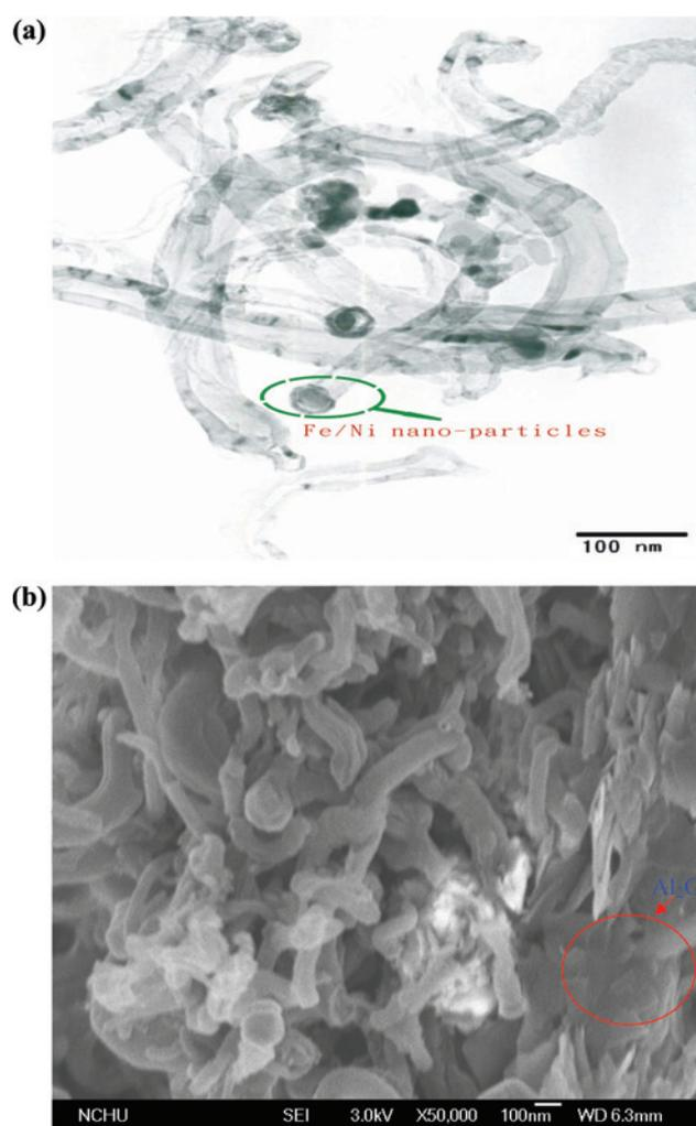
Figure 1. TEM image of CNTs on CCNTs and SEM image of aggregated CCNTs. (a) TEM image of CNTs with Fe–Ni particles on tips on CCNTs. (b) SEM image of aggregated CCNTs.
