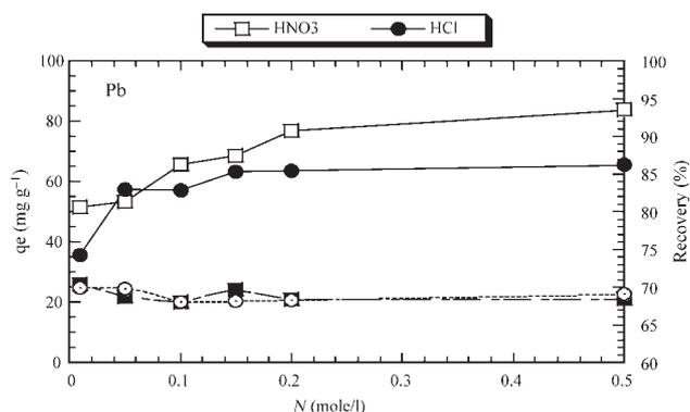
Figure 5. Recovery percentages and capacities of CCNTs with different concentrations (Normal as eq/L) of HNO<sub>3</sub> and HCl concentrations.
