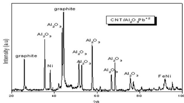
Figure 2. The XRD diagram of CCNT with no detection of adsorbed  $\text{Pb}^{2+}$  (Horng *et al.*, 2006).
