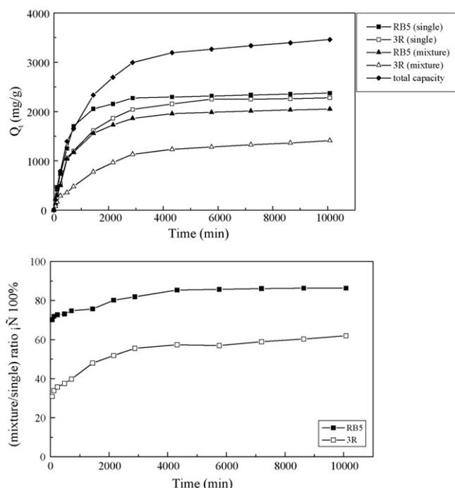
**Fig. 7.** (a) Absorption kinetics of the single and the mixture of RB5 and 3R on the ECH–RB5–NaOH microparticles (diameter: 149–250  $\mu\text{m}$ ) in 4.0 mM initial concentration of each dye at pH 3.0 and 30 °C. (b) The ratio of the adsorption capacity between the mixture solution and the single dye solution.
