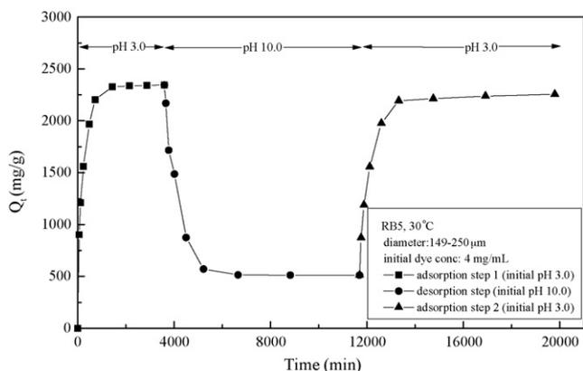
**Fig. 8.** Adsorption and desorption of RB5 dye on the ECH–RB5–NaOH microparticles (diameter: 149–250  $\mu\text{m}$ ) at 4.0 mg/mL initial concentration of dyes and 30 °C with three steps: adsorption step 1 at pH 3.0, desorption step at pH 10.0 and adsorption step 2 at pH 3.0.
