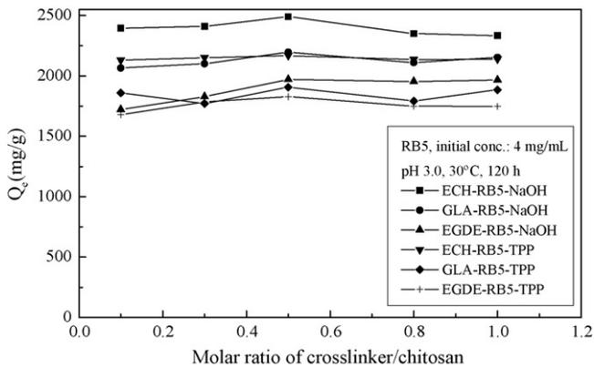
**Fig. 4.** Adsorption capacity of RB5 dye on the templated crosslinked-chitosans (diameter: 149–250  $\mu\text{m}$ ) prepared from different molar ratios of crosslinker/chitosan in 4.0 mg/mL initial concentrations of dye for 120 h at pH 3.0 and 30  $^{\circ}\text{C}$ .
