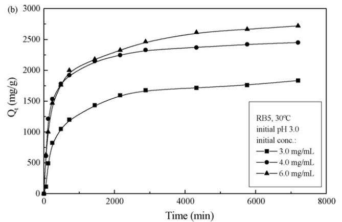
**Fig. 5.** Adsorption kinetics of RB5 dye on the ECH-RB5-NaOH microparticles (diameter: 149–250  $\mu\text{m}$ ): (a) different initial pH solutions and (b) different initial concentrations of dye.
